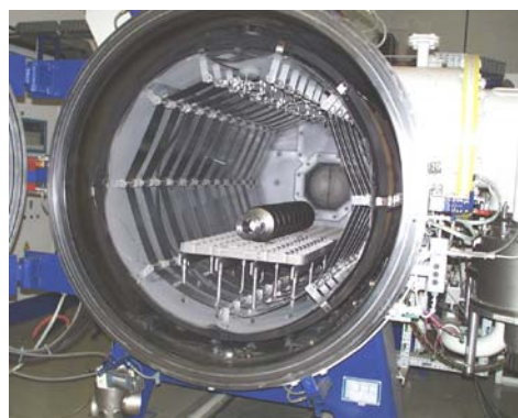
Figure 3 : Cavity loaded inside the furnace
