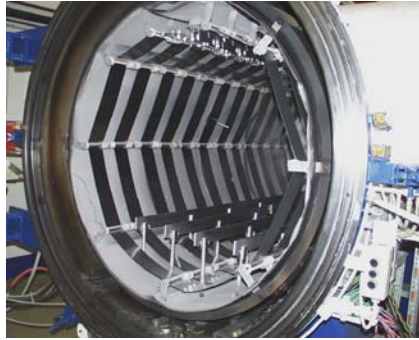
Figure 4: Rails at the bottom of the hot zone to support the bottom hearth
