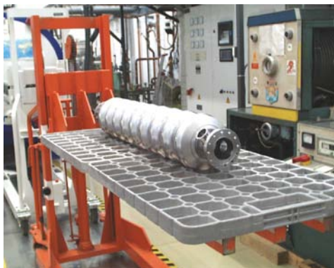
Figure 2: Cavity Loading Cart with Hearth & cavity
